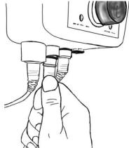
C: Make sure there are no tangles. Then plug the 24V Motor into place.
