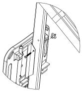
27. Attach foot rest to seat with bolts and thumbnuts.
