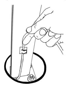
B: Lightly tension the wire and clip it into the higher mast clip.
