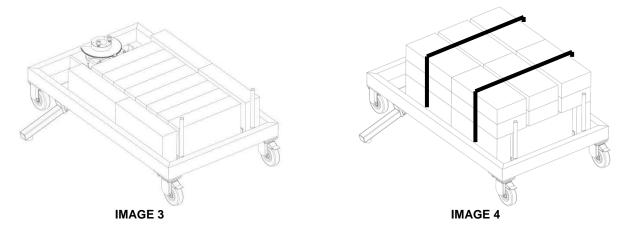
**Image 3** shows the first layer of concrete weights installed. **Image 4** shows how to properly stack the last two layers of concrete weights, using all 24 blocks. Close all gaps between the top layers, ensure they are all touching and pressed firmly together before tightening the weight straps.
