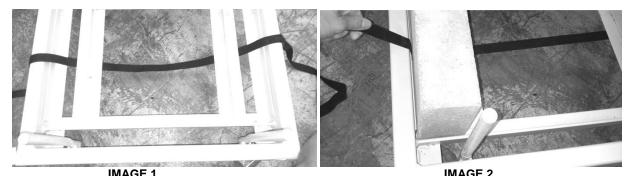
Lace the belts through the frame, as shown in **image 1**. Place the outer most blocks in position, as shown in **image 2** and pull the slack out of the restraint belts.
